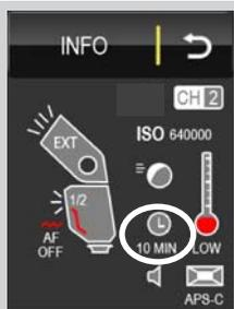
automatic unit switch-off is shown in the INFO display. The flash ready indicator ⑥ and the indicators on the LC display disappear. The ⇄ ⑦ button flashes red in stand-by mode.
